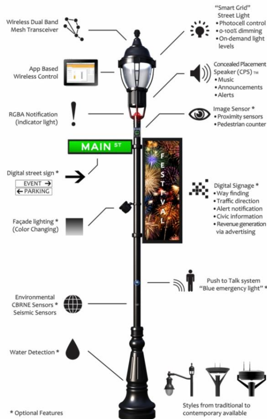
Figure 29 : Smart Street Light
